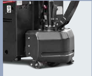
Additional wheels are equipped to have better stability
